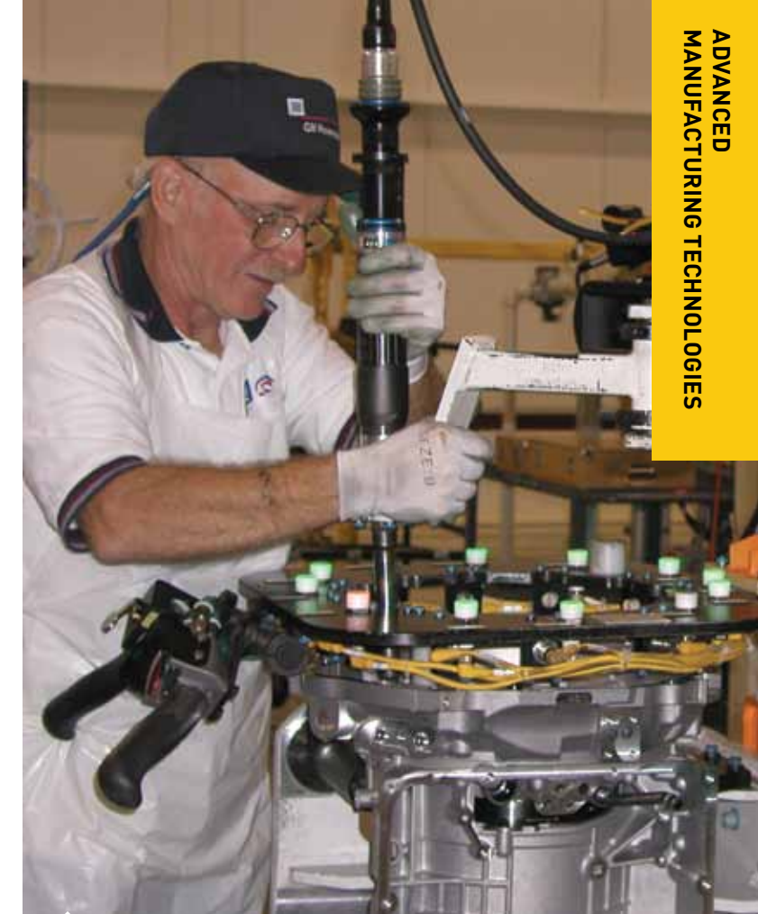
A GENERAL MOTORS BALTIMORE TECHNICIAN ASSEMBLES A 2-MODE HYBRID TRANSMISSION.
